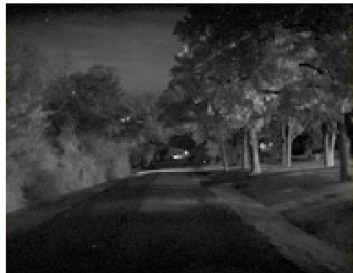
Figure 2: A comparison of nighttime images. Ambient visibility (Above). Visibility of SWIR at nighttime, no illumination (Below) **.
