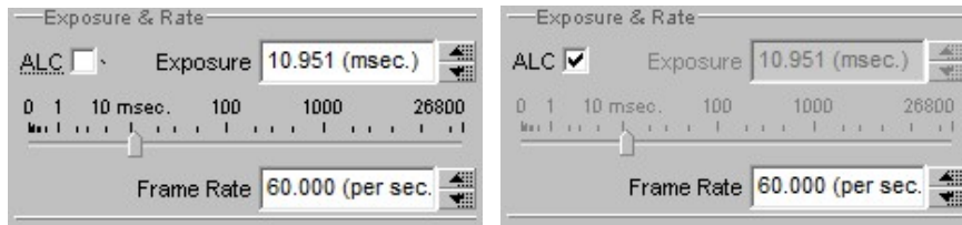
Figure 7: ALC and Manual Exposure Time Controls.
