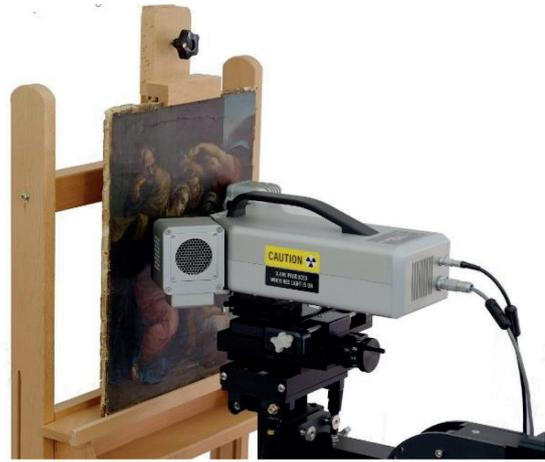
**Figure 1:** The Duetto 2 system with a Raptor CCD camera
