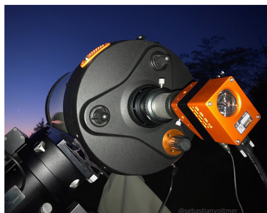
Figure 3: Tracking mount with the attached Ninox 640 II to the telescope
